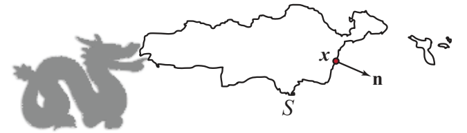
Figure 2: Flame front surface: Sound is computed by evaluating and differentiating a velocity flux integral I(t) over this dynamic surface.
